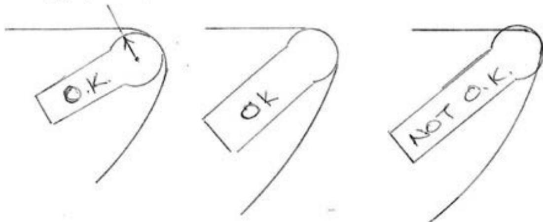
2. Leading Edge of the Runner (E.6): (10/1/2010) In Specification E.6, the 3/4" (19 mm) dimension above the ice which establishes the upper limit of the sharpened ice contact edge shall be determined according to the diagram "19 mm Dimension". Line A represents the official measurement line. (See Figure E.2: 19 mm Dimension in Specification E.6)
