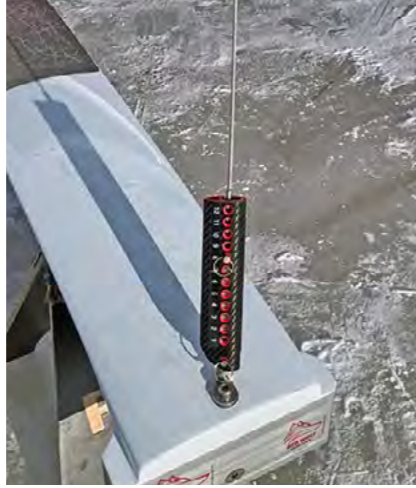
SHROUD ADJUSTER: Here's an aerodynamically shaped shroud adjuster with numbers. I suspect these are available commercially.
