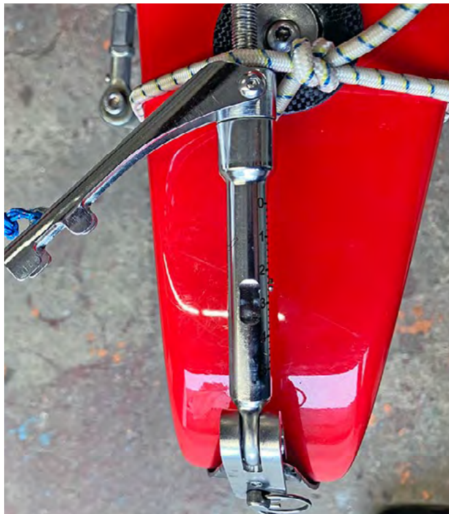
FORESTAY ADJUSTER: There was a really nice forestay adjuster on the red boat. It was expensive but nice, with numbers and its own turning mechanism so that carrying a wrench wasn't necessary.
